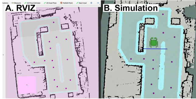
Fig. 2. Visual validation. (A) Rviz showing the waypoint sequence. (B) Simulation showing spatial coherence and costmaps.
