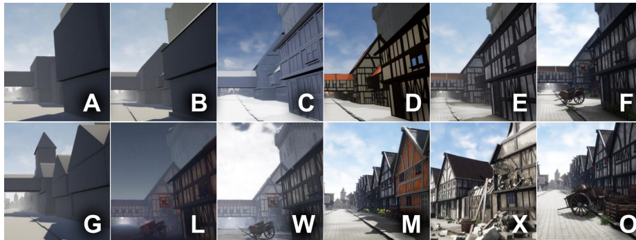
Fig. 4. The twelve level variants showing successive design stages used in this study for image analysis and correlation with Impression Curve. A - simple blockout; B - advanced blockout; C - models without materials; D - models with monochromatic materials; E - models with final materials; F - final level version; G - geometrical changes; L - lightening condition changes; W - weather changes; M - material changes; X - expression added; O - extra models added.
