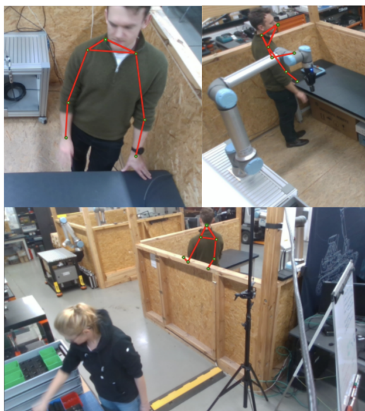
Fig. 3. Example of inaccuracies of 3D pose regression with VoxelPose (trained on considered workshop with 3 camera setup having small common field of view).
