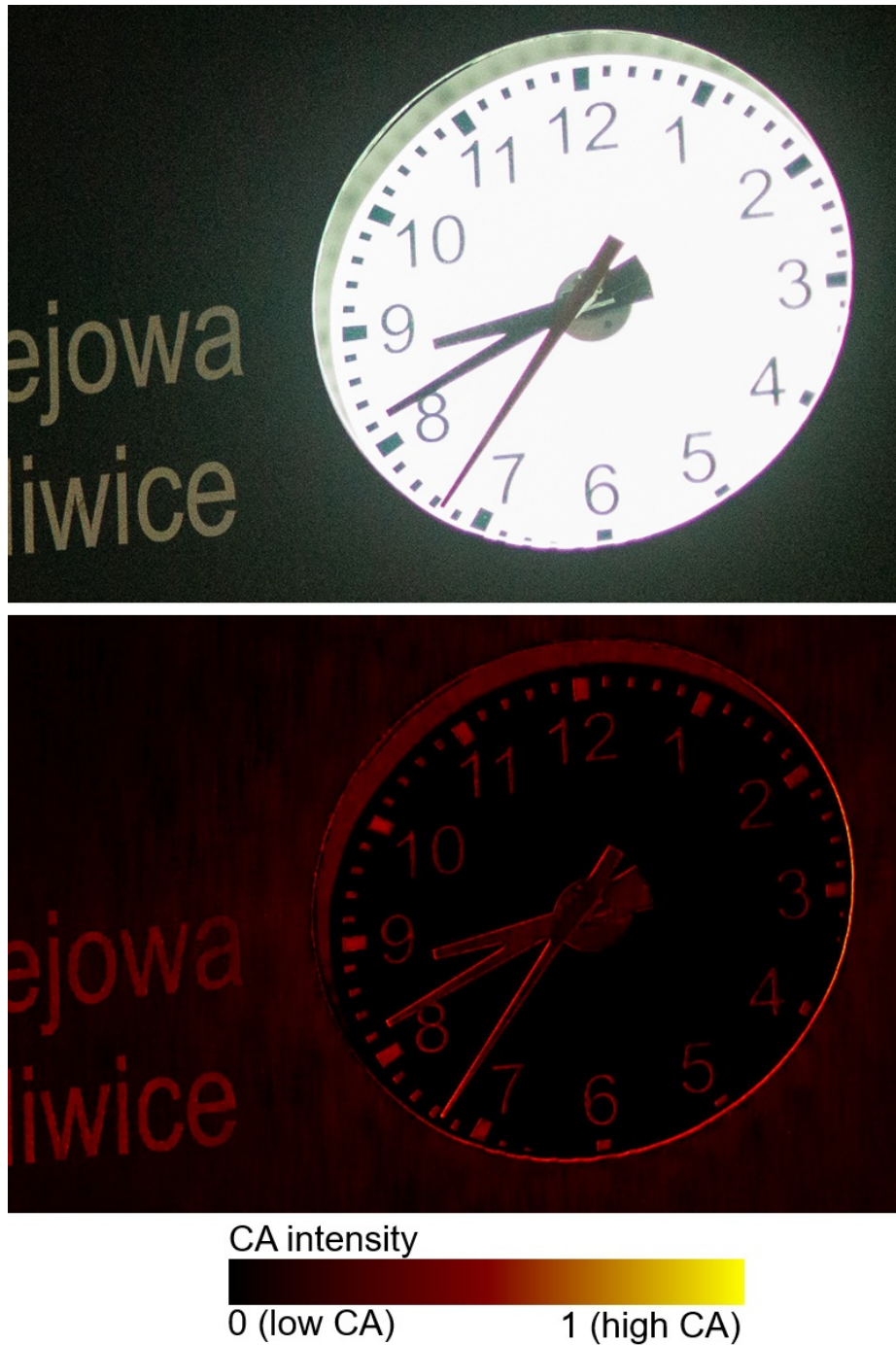
Fig. 3. Input image (top) showing visible chromatic aberration along object edges; Corresponding heatmap (bottom) of detected CA, where red-orange regions highlight areas of high aberration intensity (scale: 0–1, normalized).
