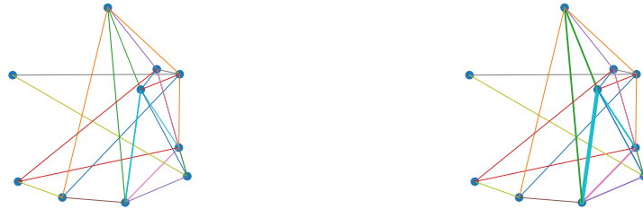
Fig. 6. Edge-dissipation redistribution in a 10-node network before (left) and after (right) optimization. Edge thickness is proportional to p_{edge,ij} = G_{ij}(v_i - v_j)^2 . The underlying topology is unchanged; effective activity attenuates couplings continuously.
