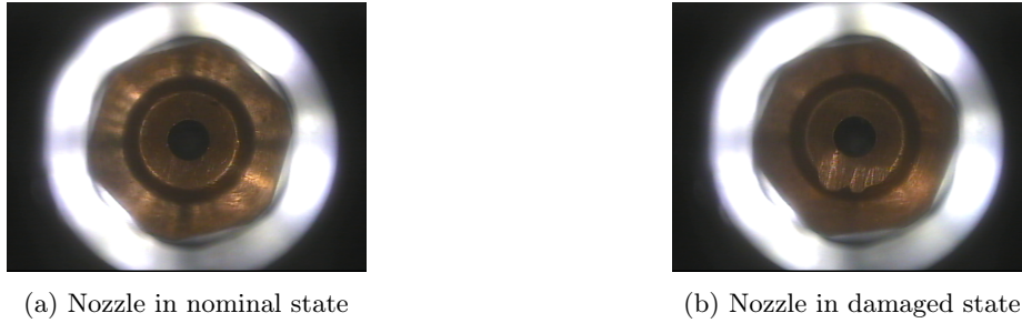
Fig. 4: Examples of cutting nozzle conditions. Images courtesy of MicroStep, spol. s r.o.
