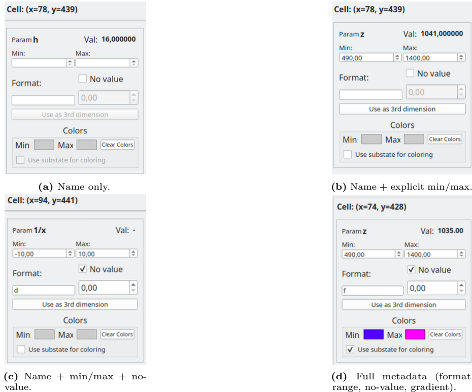
Fig. 4: Substate configuration levels supported by the visualizer. Explicit bounds stabilize colormap normalization and enable elevation mapping in 3D mode; no-value markers are excluded from rendering and range estimation.
