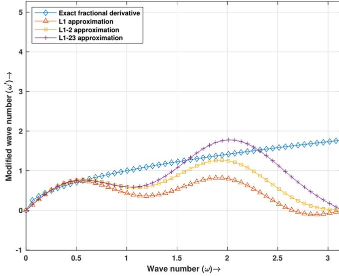
**Fig. 2.** Modified wavenumbers vs. wavenumber of difference approximations for  $J = 100$  and  $\alpha = 0.5$ .
