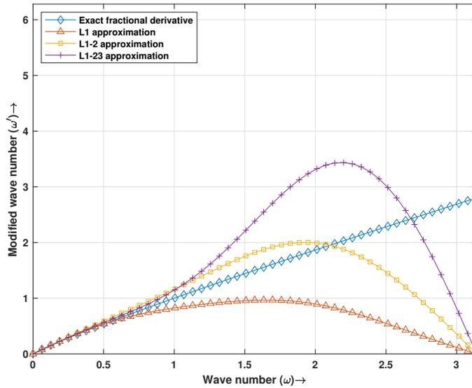
**Fig. 3.** Modified wavenumbers vs. wavenumber of difference approximations for  $J = 100$  and  $\alpha = 0.9$ .
