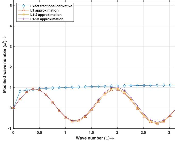
**Fig. 1.** Modified wavenumbers vs. wavenumber of difference approximations for  $J = 50$  and  $\alpha = 0.1$ .
