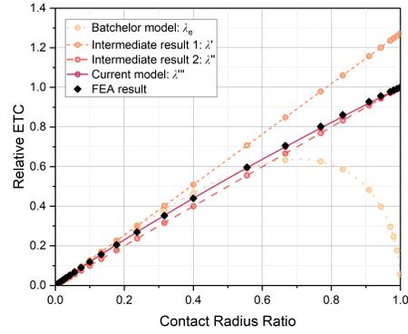
**Fig. 5.** Relative ETC results of intermediate steps and numerical model (FEA result)
