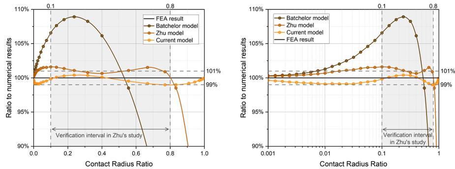
**Fig. 6.** Error analysis between numerical model (FEA results) and current model, Batchelor's model and Zhu's model in (left) linear scale (right) logarithmic scale
