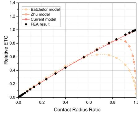
**Fig. 4.** Relative ETC results of Batchelor's model, Zhu's model, current model and numerical model (FEA result)
