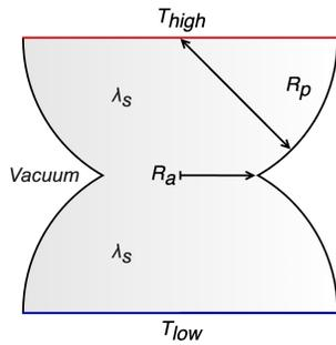
**Fig. 1.** Definition sketch of Batchelor's models and Zhu's model
