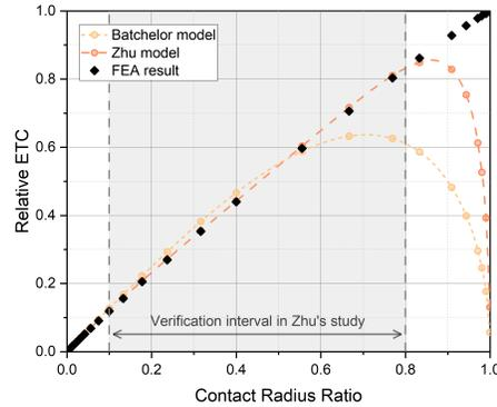
**Fig. 2.** Relative ETC of numerical model (FEA result), Batchelor's model and Zhu's model
