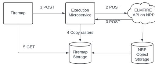
Fig. 2: Fire Simulator Workflow for Executing Fire Models on a Kubernetes Cluster
