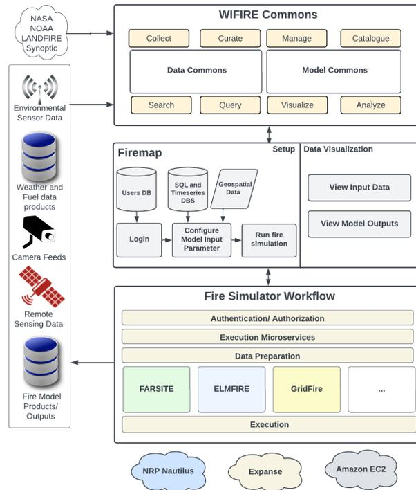
Fig. 1: Firemap’s Architecture and Workflows integrate a suite of open-source fire modeling tools with multimodal input data and user-provided parameters.
