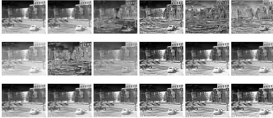
Fig. 5. Example outdoor IR image (top-left) and its variants processed using 9 color maps (in the order from Fig. 3) and then by 8 standard image processing techniques.
