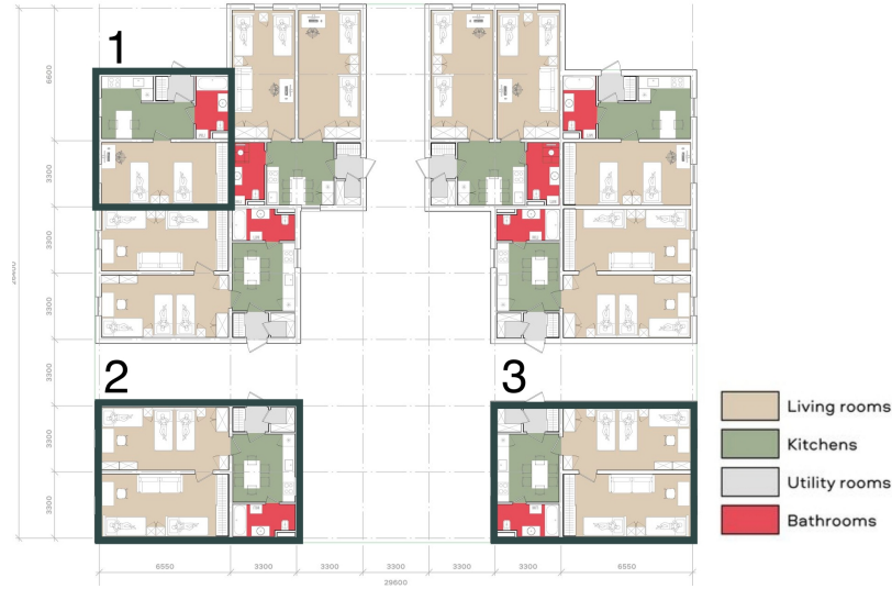
Fig. 1. The RE:Ukraine Housing project: the family arrangement type and 1-3 identified types of standard layouts.
