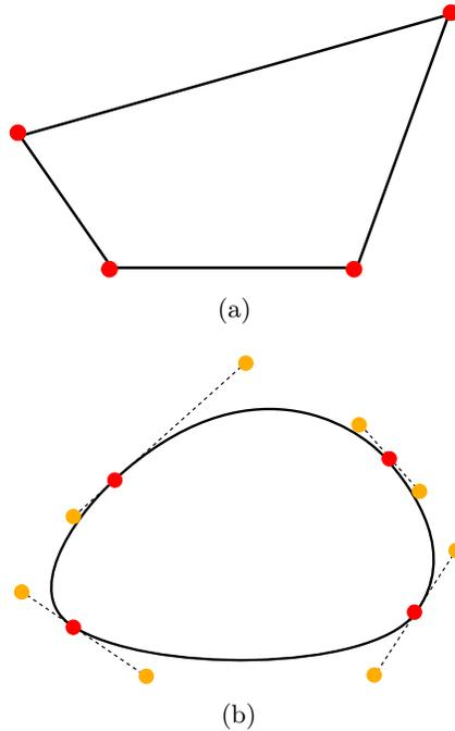
Fig. 1: The way of modeling in PIES: a) polygonal shape, b) curved shape.
