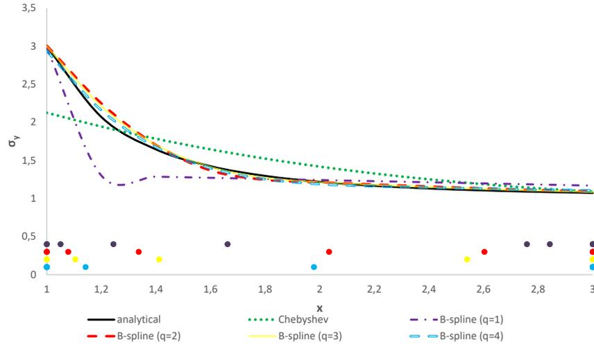
Fig. 7: Solutions  $\sigma_y$  for various degrees of B-spline functions.
