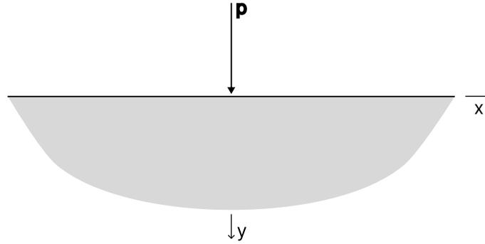
Fig. 3: A half-space with a concentrated boundary condition.
