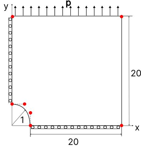
Fig. 6: The plate with a circular hole.
