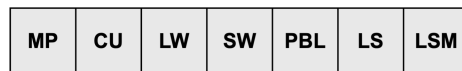
Fig. 2. Schematic representation of an individual, where each physics scheme act as “gene”. Here MP, CU, LW, SW, PBL, LS, and LSM refer to microphysics, cumulus, longwave radiation, shortwave radiation, Planetary Boundary Layer, Land Surface Model, and Surface physics schemes, respectively
