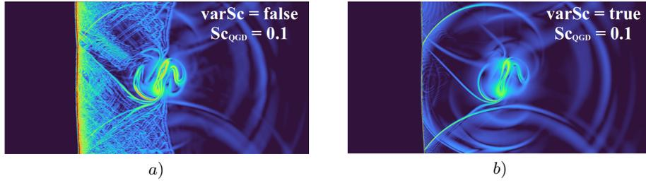
**Fig. 7.** Numerical Schlieren in QGD AMReX on a 1/1600 mesh with  $\alpha = 0.1$  and  $Sc_{QGD} = 0.1$ ,  $t_{end} = 0.7s$  : a) Dynamic Schmidt - **off**; b) Dynamic Schmidt - **on**,
