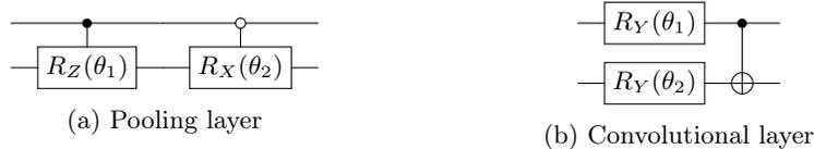
Fig. 4: Description of the convolutional and pooling layers used in our algorithm. At the end of the pooling layer we trace out the control qubit in order to reduce the dimension.
