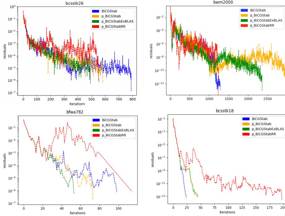
Fig. 2: Residual history of the four BiCGStab-like methods;  $tol = 10^{-13}$ .
