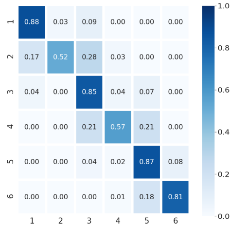
Fig. 4. Confusion matrix for VGG19 convolutional neural network for structure form classification
