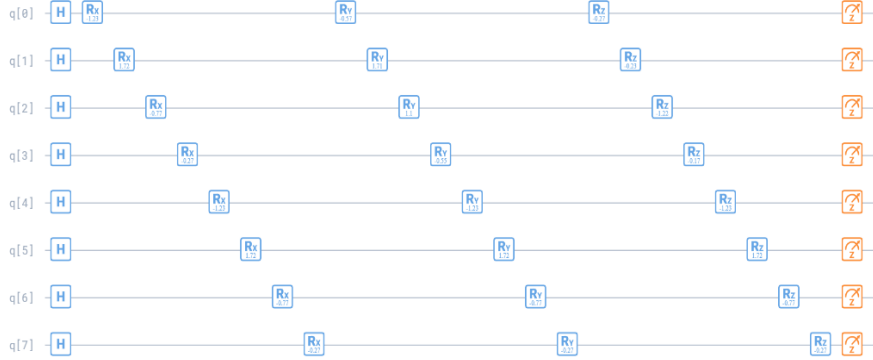
Fig. 2. A diagram of the quantum evolution circuit at Quantum Inspire platform.
