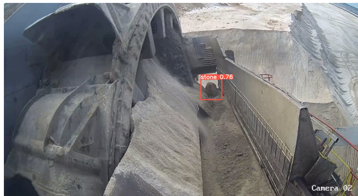
Fig. 1. Camera view with a visible stone on the conveyor belt
