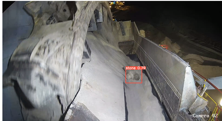
Fig. 2. Camera view with a visible stone on the conveyor belt (artificial light)
