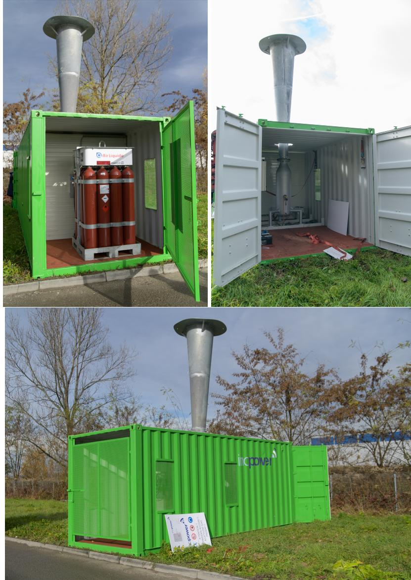
Fig. 2: Hail cannon: Container with acetylene cylinders and control panel. Combustion chamber with the conical outlet pipe.
