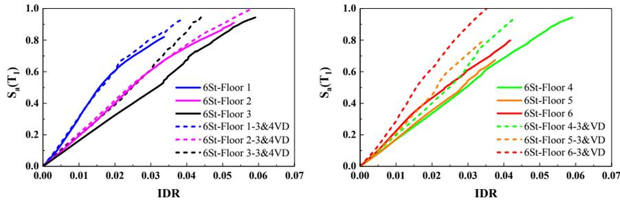
**Fig. 6.** Comparison between IM-IDA curves of all floor levels of the 6-story colliding SMRF retrofitted with two linear VDs in third and fourth story levels, subjected to NPL record subset given clear distance of 0.298 m.
