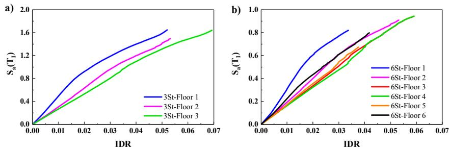
**Fig. 3.** IM-IDA curves of all floor levels of the 3-, and 6-story colliding SMRFs subjected to NPL record subset given clear distance of 0.298 m.
