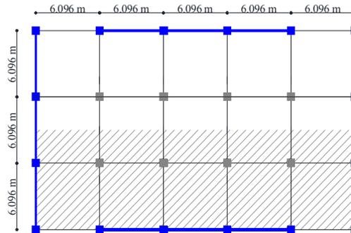
Fig. 2. Structural plan of the 3-, and 6-story SMRFs.
