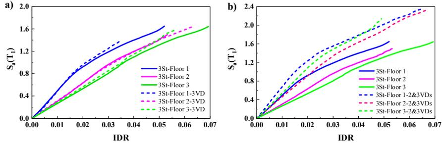
**Fig. 4.** Comparison between IM-IDA curves of all floor levels of the 3-story colliding SMRF retrofitted with, a) one linear VD in third story level, b) two linear VDs in second and third story levels, subjected to NPL record subset given clear distance of 0.298 m.
