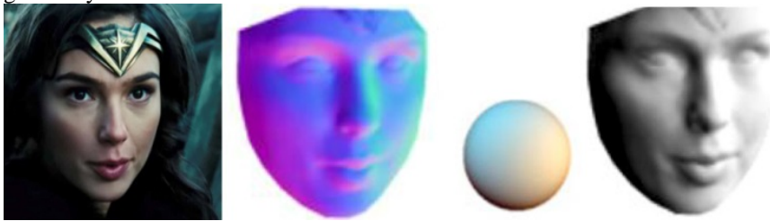
Fig. 1. Shape-from-shading based reconstruction: input image, estimated normal map, and rendered model (from left to right) [15].
