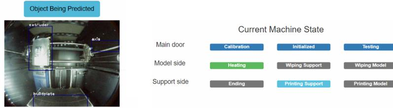
Fig. 6. Machine state predictions as shown on GUI
