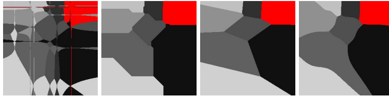
Fig. 1: Voronoi diagrams for various distance measures \rho_p , p = 1/4, 1, 2 and 4 , from left to right. N = 8 (for improved visibility the Voronoi cells have different colors, in spite of the fact that we examine a dichotomy problem, i.e. the binary classifiers only)
