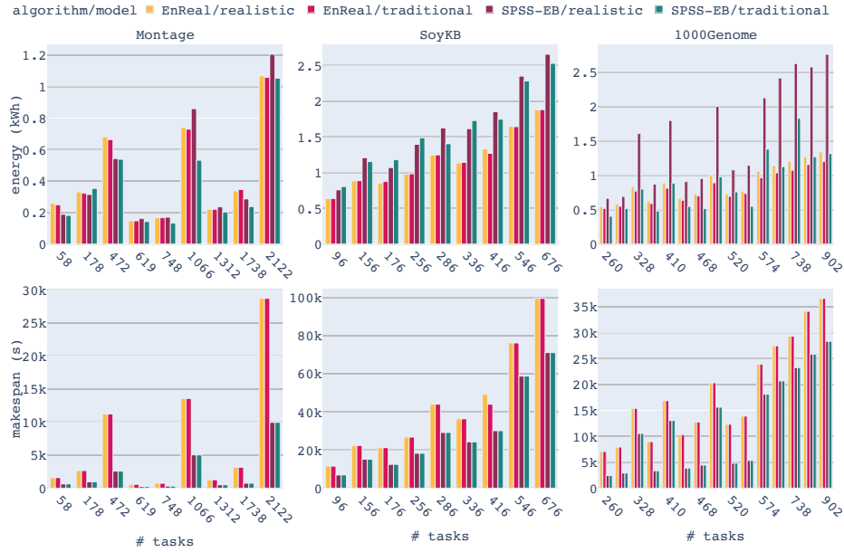
Fig. 1. Simulated workflow energy consumption (top) and makespan (bottom) for each workflow application instance for the SPSS-EB and EnReal algorithms. Results are shown when simulating energy consumption with the traditional power model and the realistic power model.
