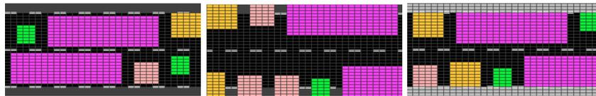
**Fig. 2.** A traffic jam without a corridor of life (top), with corridor of life (in the middle), and with corridor of life on the road with curbs (bottom)
