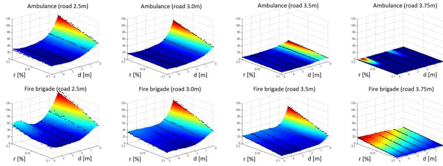
**Fig. 3.** Ambulance (the first row) and fire brigade (the second row) delays on the road with two lanes (a) 2.5m wide each, (b) 3.0m wide each, (c) 3.5m wide each, and (d) 3.75m wide each, depending on the road density -  $r$  and distance between vehicles -  $d$ .
