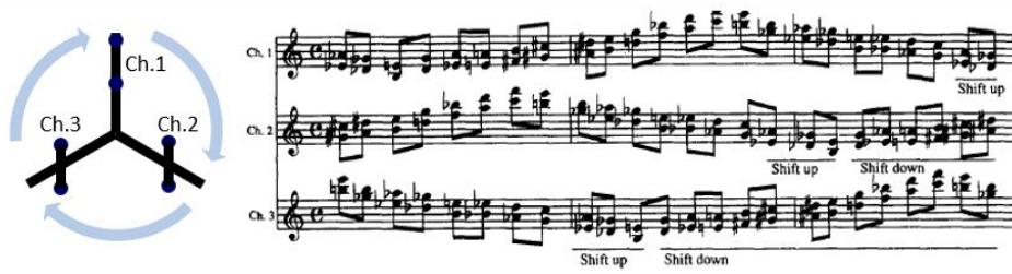
Fig. 3. In this example, each leg of the tripod on the left, is represented on the right by two voices in a musical mapping. A variation on Bresenham’s circle drawing algorithm is used to rotate the tripod and to generate musical information.
