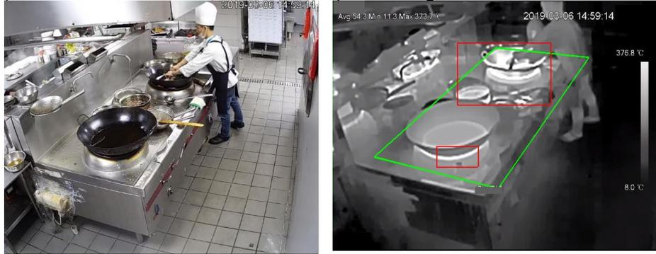
Fig. 3. Optical video (left) and thermal video (right) of the same site. The temperature measurement locations are annotated as red boxes.
