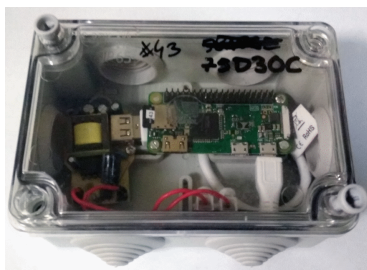
Fig. 3. The Hub in IP57 enclosure
