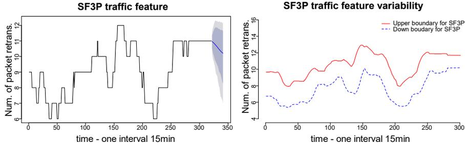
**Fig. 7.** Railway PLC sign traffic feature SF3P (number of packet retransmissions) neural network prediction intervals (20 samples horizon) with narrower (80%) and wider (90%) prediction intervals (on the left) and SF3P traffic feature variability used for model calculation (on the right).
