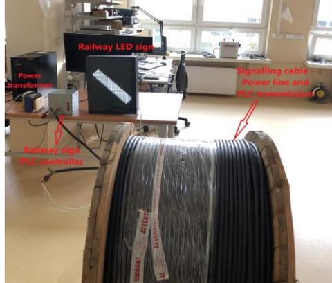
**Fig. 4.** Part of experimental testbed used for measurements and methodology verification representing connections between main elements of railway PLC signs together with power and transmission line (1 km length).
