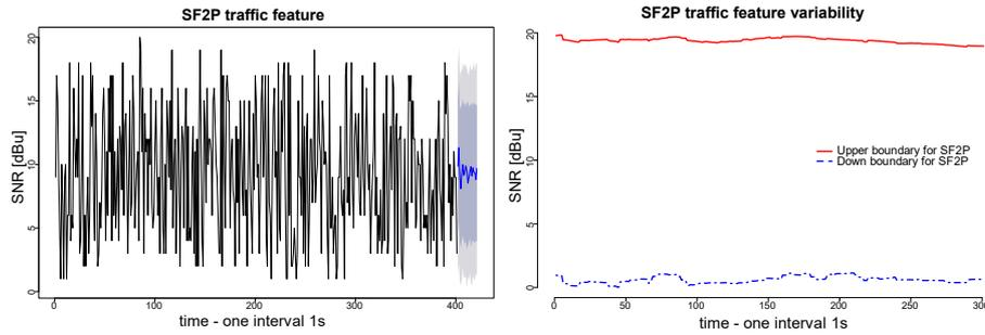
**Fig. 6.** Railway PLC sign traffic feature SF2P (SNR [dBu]) neural network prediction intervals (20 samples horizon) with narrower (80%) and wider (90%) prediction intervals (on the left) and SF2P traffic feature variability used for model calculation (on the right).
