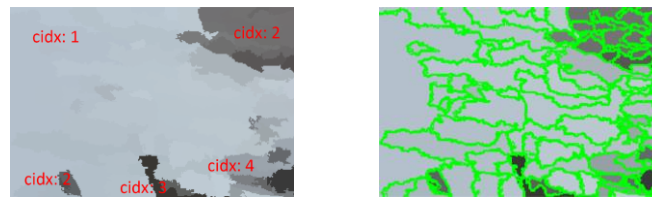
Fig. 3. Comparison of mosaic appearance (4 main colors - cidx ) (left) and imposed limits after binarization (right).
