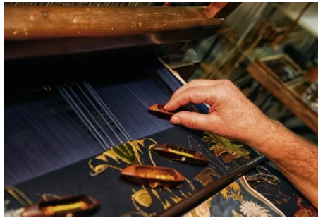
Fig. 1. Making a Valencian espolín with a Jacquard loom. It can be seen how the golden threads do not go from side to side of the fabric, but remain concentrated around the pictorial motifs.
