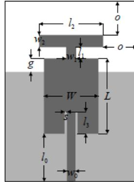
**Fig. 2.** Geometry of the dual-band patch antenna.
