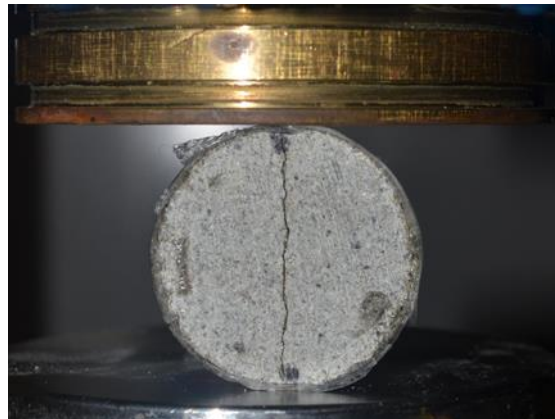
Fig. 2. Fracture creation using the Brazilian test procedure.
