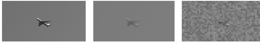
Fig. 1. Example of good quality measurement (left), low contrast measurement (center), and measurement of the noisy low contrast (right) for the aircraft.
