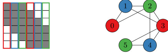
Fig. 1: Sparsity pattern of the Hessian (left) and the corresponding adjacency graph (right) with colors obtained by acyclic coloring for the function from (6)
